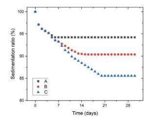
Figure 14 - The sedimentation ratio as a function of time for the three MRF, visually measured through the sediment height method. The test tubes were under rest, at normal gravity and room temperature  $(20 \pm 5 \text{ °C})$ .
