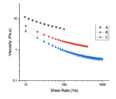
Figure 10 - Viscosity curves (off-state) of each MRF.
