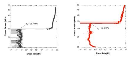
Figure 11 - On-state yield stress curve of fluid A.
