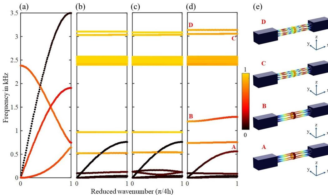
FIG. 2. The phononic dispersion curves along the  $x$ -direction in the first Brillouin zone ( $\Gamma X$ ) for the four beams. (a) The homogeneous medium cell. (b) The nonchiral isotactic cell. (c) The chiral isotactic cell. (d) The chiral syndiotactic cell. (e) Screenshots of the syndiotactic chiral cell beam's eigenmodes at points A, B, C, and D.
