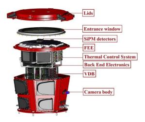
Fig. 1 Exploded 3D layout of the ASTRI-Horn camera.
