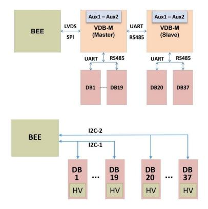
Fig. 7 VDB architectures for the ASTRI-Horn (above) and Mini-Array (below) cameras.
