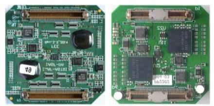
Fig. 4. Comparison of the ASIC boards (50mm × 50mm); on the left the ASTRI-Horn configuration, on the right the one adopted for the cameras of the ASTRI Mini-Array.
