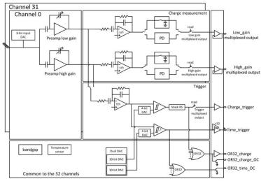
Fig. 3. Citiroc ASIC block diagram.
