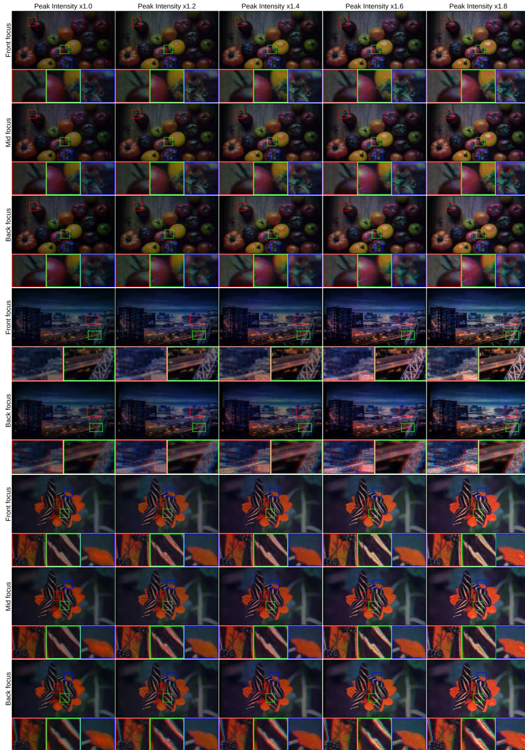
Fig. 8. Three dimensional scenes using our multi-color holograms. Photographs show a multiplane image generated by our multi-color hologram scheme with three focus planes. The targeted brightness level is \times 1.8 . (150 ms exposure time)
