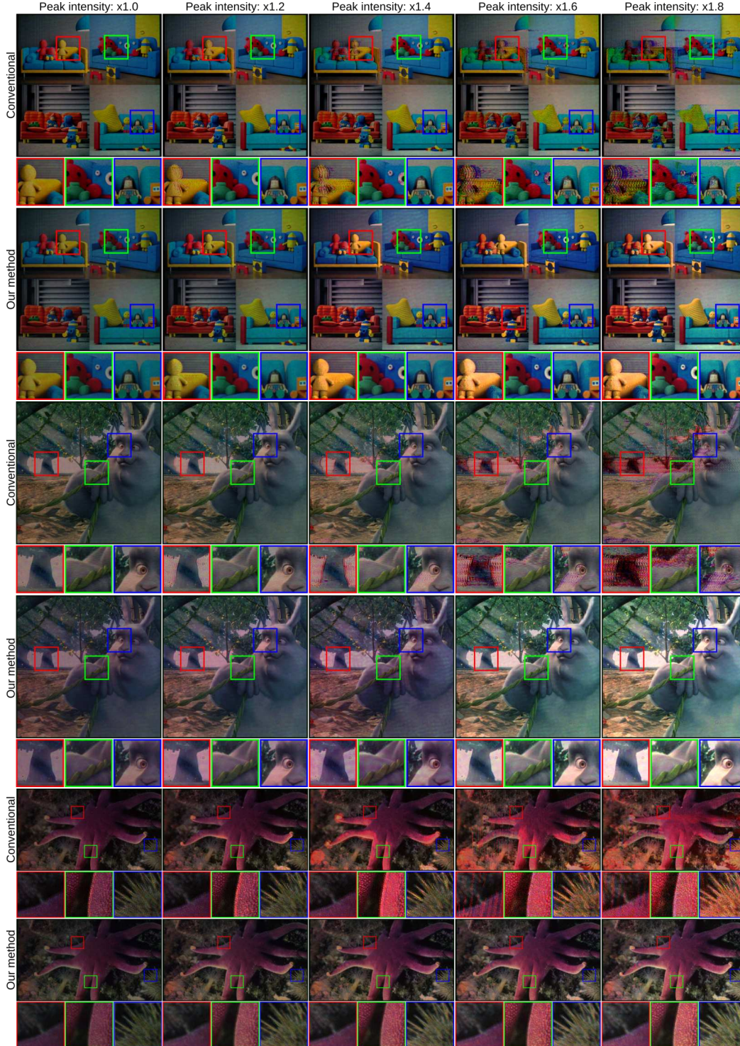
Fig. 3. Increasing peak brightness levels with our multi-color holograms. Photographs show that our method can enhance the peak brightness levels of the captures up to \times 1.8 without artifacts or distortions. In contrast, the conventional hologram fails to support beyond \times 1.0 (140 ms exposure).
