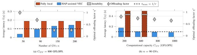
Fig. 1: Optimal offloading factor  $\eta^*$  (right axis) and average latency  $\bar{t}(\eta)$  (left axis) vs. n and  $C_{GV}$ , for r = 10 fps and  $n_{UL} = 3$  Mb. Striped bars are interrupted to represent the case of unstable queues where the latency increases indefinitely in the long term.
