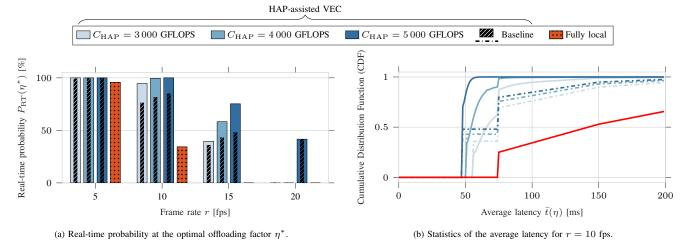
Fig. 2: Real-time probability (left) and average latency (right) vs.  $C_{\text{HAP}}$  and r, when  $C_{\text{GV}} = 800$  GFLOPS, n = 100 GVs and  $n_{\text{UL}} = 1$  Mb. Dash-dot lines and black striped bars refer to a baseline offloading scheme which balances the load of the HAP and of the GVs equally.
