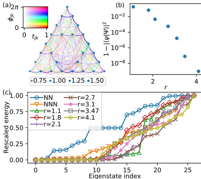
FIG. 5. The properties of the nonlocal Hamiltonians constructed for an  $M = 6$  target state. (a) The hoppings and onsite potentials of the  $r = 4.1$  Hamiltonian. (b) The error of the approximation of the model state by the ground state of the Hamiltonians, as a function of radius  $r$ . The error is defined as one minus the squared overlap. (c) The single-particle energy spectra of various Hamiltonians, showing the emergence of a flat “band” for high  $r$ .
