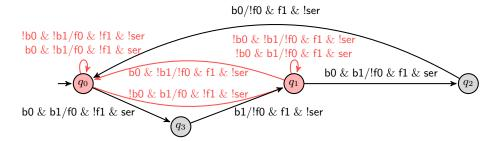
Fig. 7: Mealy machine returned by our tool on the elevator specification with additional examples. The preMealy machine obtained after generalizing the examples and before completion is highlighted in red. This took 3.10s to be generated.
