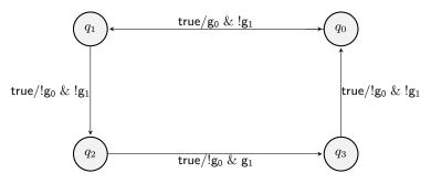
Fig. 13: Mealy Machine for No Subsequent Grants returned by Strix
