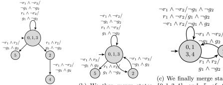
(a) We then merge states  $\{0,1\}$  and 3 of the pre-Mealv machine PTA, i.e., we merge classes  $[\epsilon]$ and  $[\{\neg r_1 \land \neg r_2\}\{\neg g_1 \land$  $\neg g_2\} \# \{r_1 \land \neg r_2\} \{g_1 \land \neg g_2\}].$ We then check for PTA - realizability which is found to be true. The resulting machine is shown here.
