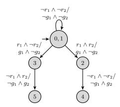
(a) We begin by merging states 0 and 1 of the preMealy machine PTA, i.e., we merge classes  $[\epsilon]$  and  $[\{\neg r_1 \land \neg r_2\}\{\neg g_1 \land \neg g_2\}]$ . We then check for PTA – realizability which is found to be true. The resulting machine is shown here.
