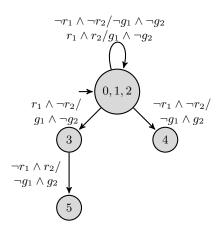
(b) We then proceed by merging states  $\{0, 1\}$  and 2 of the preMealy machine PTA, i.e., we merge classes  $[\epsilon]$  and  $[r_1 \wedge r_2/g_1 \wedge \neg g_2]$ . We then check for PTA – realizability which is found to be false. We corraborate by observing the trace  $(r_1 \wedge r_2/g_1 \wedge \neg g_2)^{\omega}$  does not satisfy the LTL subformula  $G(r_2 \implies Fg_2)$ . Thus the merge is unsuccesful and is reversed.
