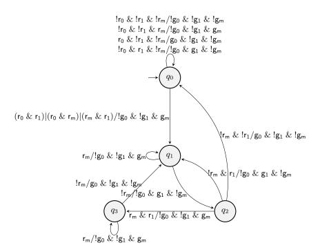
Fig. 11: Preliminary machine obtained by our tool (without additional examples) on the Prioritized Arbiter specification
