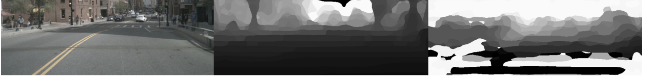
Figure 9: Depth estimation results. From left to right: original FRONT camera images, BEVDepth (Li et al., 2022a) depth prediction results, BEVDet (Huang et al., 2021) depth prediction results. Accurate depth estimation provides the model with strong robustness.
