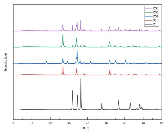
Fig. 1 XRD patterns for samples of pure ZnO (black line), pure  $SnO_2$  (red),  $ZnO:SnO_2 = 1:1$  (blue line),  $ZnO:SnO_2 = 1:2$  (green line), and  $ZnO:SnO_2 = 2:1$  (purple line).
