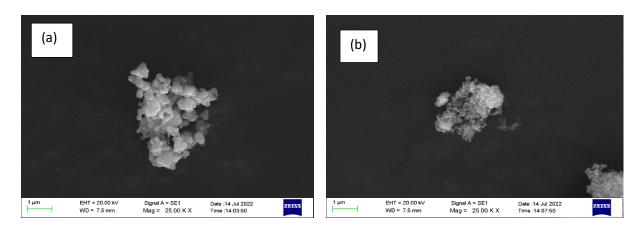
Fig. 2 SEM images of the nano particle samples (a) pure ZnO (b) pure SnO<sub>2</sub> at a 25.00k magnification
