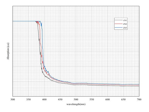
Fig. 4 Absorption spectra of the  $ZnO:SnO_2 = 1:1$  (black line),  $ZnO:SnO_2 = 1:2$  (red line), and  $ZnO:SnO_2 = 2:1$  (blue line).
