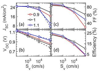
**FIG. 4**. Effect of interface recombination velocity  $(S_v)$  on the performance metrics of PSC for different ion migration cases (immobile ion density of  $5 \times 10^{17} cm^{-3}$ ,  $G = 5.21 \times 10^{21} cm^{-3}/s$ ).
