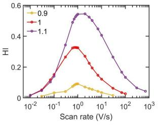
**FIG. 6.** Hysteresis vs. scan rate for different ratios of ions in the perovskite layer. All devices have immobile ion density of  $4 \times 10^{17} cm^{-3}$ , ion mobility of  $10^{-10} cm^2 V^{-1} s^{-1}$ ,  $S_v = 10^2 cm/s$ , bulk SRH carrier lifetime of  $\tau_{SRH} = 10^{-7} s$  and are under uniform generation,  $G = 5.21 \times 10^{21} cm^{-3}/s$ .
