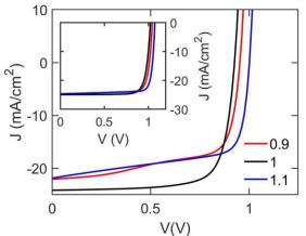
**FIG. 3**. J-V characteristics of PSC with different ion migration cases under illumination ( $G = 5.21 \times 10^{21} \text{ cm}^{-3}/\text{s}$ ) with  $S_v = 10^4 \text{ cm}/\text{s}$ . Inset shows J-V characteristics of device with  $S_v = 10^2 \text{ cm}/\text{s}$ . f = 1 indicate balanced ion case, f = 1.1 denotes case (ii) and f = 0.9 represents case (iii). All devices have immobile ion density of  $5 \times 10^{17} \text{ cm}^{-3}$ .
