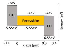
**FIG. 1.** Schematic diagram of Perovskite solar cell with energy alignment of materials.
