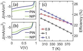
**FIG. 5.** J-V Characteristics of device with different illumination scheme for (a) f = 1.1, (b) f = 0.9 ( $S_v = 5 \times 10^4 \text{ cm/s}$ ). (c). Effect of temperature on the efficiency of Perovskite solar cells under uniform generation ( $G = 5.21 \times 10^{21} \text{ cm}^{-3}/\text{s}$ ), and  $S_v = 10^2 \text{ cm/s}$ . Immobile ion density of  $5 \times 10^{17} \text{ cm}^{-3}$  is considered for all devices.
