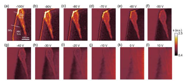
FIG. 2 The nano-IR imaging data of ABA-TLG and ABC-TLG at various gate voltages. The voltages marked here correspond to  $V_g$  -  $V_{CN}$ . The dashed lines in panel (a) mark the directions for extracting the line profiles shown in Fig. 3. The nano-IR amplitude signals plotted here are normalized to that of the SiO<sub>2</sub>/Si substrate.
