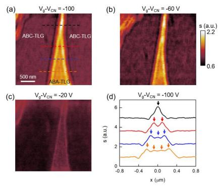
FIG 5. (a)-(c) Nano-IR imaging data of a sample area containing an ABC/ABA/ABC TLG junction at various gate voltages. (d) Line profiles extracted along the dashed lines in panel (a). The arrows mark the resonant peaks in the profiles.
