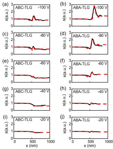
FIG. 3. Plasmon fringe profiles of ABC-TLG and ABA-TLG at various gate voltages ( $V_g$ - $V_{CN}$ ). The black curves are experimental line profiles taken perpendicular to sample edges (along white dashed lines) of the nano-IR images in Fig. 2. The red curves are the fitting profiles using a quantitative s-SNOM model [14,19,21]. The nano-IR amplitude signals in the profiles are normalized to that of the SiO<sub>2</sub>/Si substrate.
