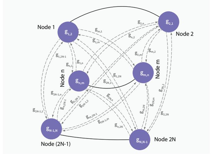
Fig. 2. Graph representation of a flexible duplex network. Solid lines indicate  $e_d$  and dashed lines indicate  $e_i$ , where  $g_{i,j} = |h_{i,j}|^2$  and  $m = 2(n \bmod 2) + n - 1$ .
