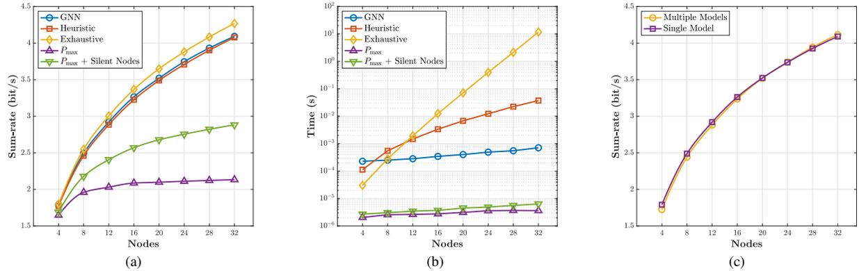
Fig. 4. (a) Average sum-rate comparison of different algorithms. (b) Running time per sample for different algorithms. (c) Sum-rate comparison of a set of models (multiple models) which are trained with a fixed number of nodes and a model (single model) trained with a variable number of nodes.
