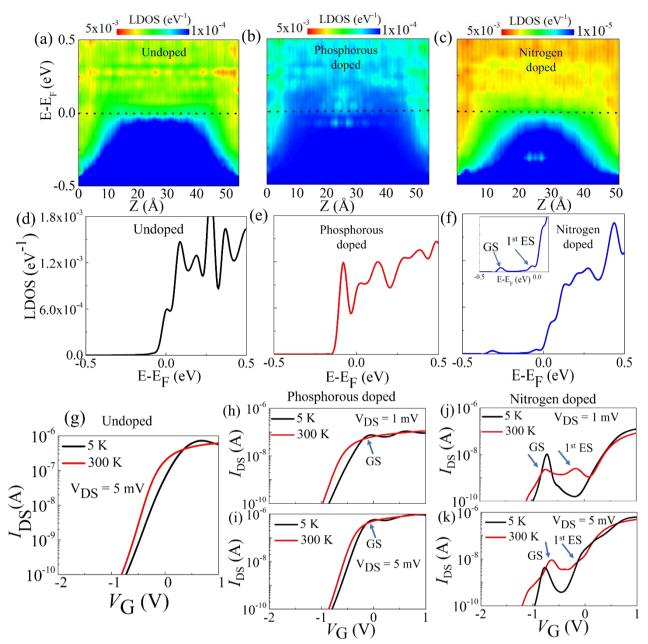
Figure. 5: (a-c) LDOS spectra of an undoped, P-doped, and N-doped silicon nanowire transistor, respectively. (d-f) LDOS spectrum at z = 26.93 Å for undoped, P-doped, and N-doped silicon nanowire transistor, respectively. Inset of Fig. 5(f) indicates the zoom in spectrum, exhibiting the GS and and 1<sup>st</sup> ES of N-donor. Simulated  $I_{DS}-V_G$  characteristics for (g) undoped, (h-i) P-doped, and (j-k) N-doped devices.
