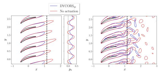
(d) Average total pressure contour around the blades and total (e) Instantaneous vorticity contour for the case without acpressure profiles at the downstream measurement location for the case without actuation and the case using  $DYCORS_{ip}$ .
