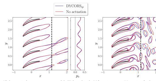
(d) Average total pressure contour around the blades and total pressure profiles at the downstream measurement location for the case without actuation and the case using G-DYCORS<sub>*ip*</sub>.
