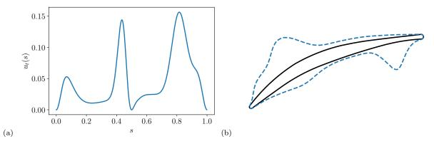
Figure 5: Example of a representative actuation. (a) presents the tangential velocity as function of the arc-length s while (b) shows the actuation (solid blue line) superposed to the blade profile (black dashed line).
