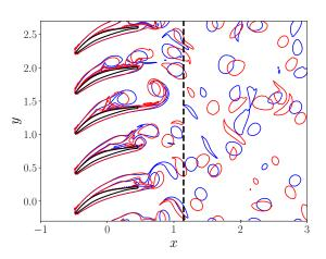
(d) Average total pressure contour around the blades and total pressure profiles at the downstream measurement location for the case without actuation and the case using G-DYCORS $_{ip}$ .
