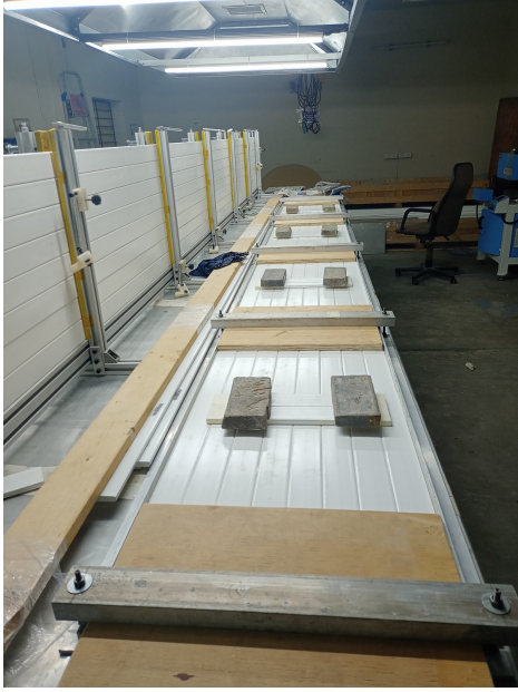
Figure 3: Di-counters glued and clamped to an Al plate for tile fabrication.
