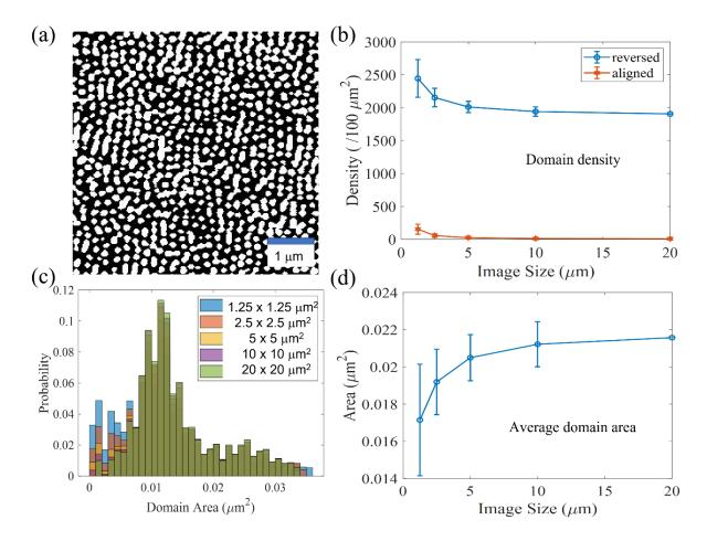
FIG. 3. Results for a predominantly **bubble pattern**. (a) Close-up view from a 20 x 20  $\mu$ m<sup>2</sup> MFM image (binarized); (b) Density of white domains  $\rho_w$  and black domains  $\rho_b$ , as function of the image size *L* it is estimated on; (c) Distribution of domain areas for the reversed (white) domains for various partition sizes *L*. The bin size is 0.001  $\mu$ m<sup>2</sup>; (d) Averaged domain area as function of the image size *L*.
