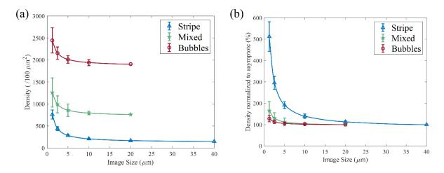
FIG. 4. Comparative plots for the stripe, mixed and bubble states. (a) Density  $\rho_w$  of reversed domains as function of the image size *L* it is estimated on, with interpolated curves; (b) Same density curves, normalized to their asymptotic value for comparison purposes.
