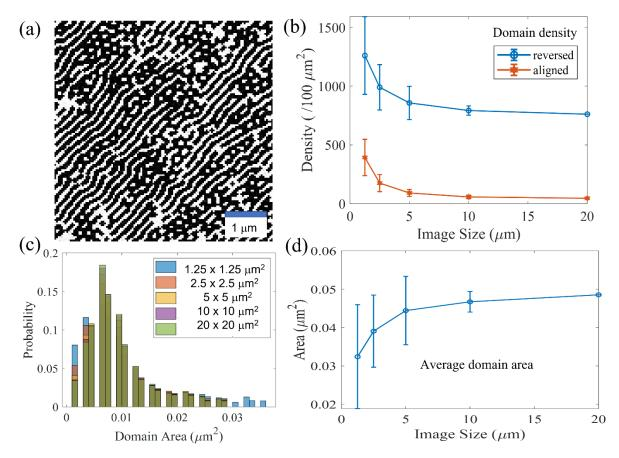
FIG. 2. Results for a **mixed stripe-bubble pattern**. (a) Close-up view from a 20 x 20  $\mu$ m<sup>2</sup> MFM image (binarized); (b) Density of white domains  $\rho_w$  and black domains  $\rho_b$ , as function of the image size *L* it is estimated on; (c) Distribution of domain areas for the reversed (white) domains for various partition sizes *L*. The bin size is 0.001  $\mu$ m<sup>2</sup>; (d) Averaged domain area as function of the image size *L*.
