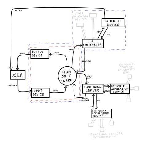
Figure 5: Data flow diagram for the typical virtual assistant hub in the home
