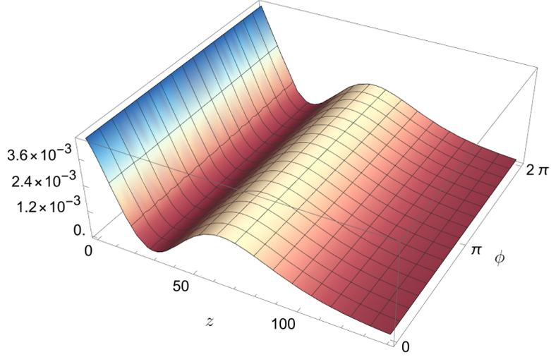
Figure 2: Normalized probability density  $\mathcal{P}$  as a function of the coordinates  $(\phi, z)$  for a nanoscroll geometry with parameters  $N = 5$ ,  $R = 5$ ,  $D = 100$ ,  $g = 10^{-3}$ ,  $\alpha = 2 \times 10^{-2}$ ,  $v_0 = 200$ ,  $w_0 = 100$ .
