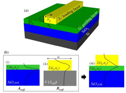
**Figure 1. (a)** Schematic of the hybrid optical waveguide. **(b)** The weakly-confined vertical mode profiles in the (i) loading and (ii) guiding layers of the hybrid waveguide are shown with dotted black lines. The right image (iii) shows the confined mode formed by combining these weakly-confined vertical optical modes.
