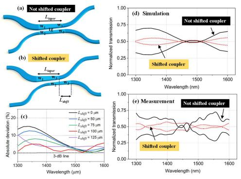
**Figure 6.** Ultra-broadband 3-dB directional coupler. Schematic of the (**a**) not shifted coupler, i.e.  $L_{shift} = 0$  (**b**) the shifted coupler  $L_{shift} > 0$ . (**c**) Absolute deviation from 50/50 coupling ratio for different  $L_{shift}$  values. Note that for  $L_{shift} = 100 \,\mu\text{m}$ , the deviation gets smaller. (**d**) Simulation and (**e**) measurement results of the not shifted ( $L_{shift} = 0$ ) coupler and shifted ( $L_{shift} = 100 \,\mu\text{m}$ ) coupler.
