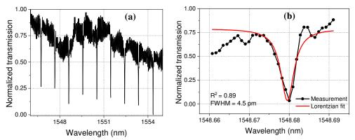
**Figure 4. (a)** Transmission measurement results of the fabricated elliptical ring resonator using a broadband light source and OSA. **(b)** The measurement of the resonance peak at 1548.68 nm using a tunable laser and photodetector. Redline is the Lorentzian fit of the experimental data.
