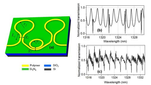
Figure 7. (a) Schematic FP-ring structure. (b) The FDTD simulation results and (c) the transmission measurement results. Due to memory limitations, the radii of the microring resonators were chosen smaller than the fabricated devices (i.e.  $50 \mu m$ ). Except for the FSR difference, the spectra represent the behavior of the device very well.
