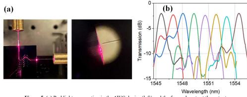
Figure 5. (a) Red light propagation in the AWG device (left) and the focused spots at the output channels (right). (b)Transmission measurement results of the fabricated AWG device.
