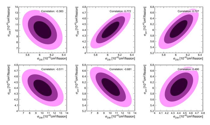
FIG. 5. Isotopic IBD yield contours for a combined fit of hypothetical HEU, LEU, and RG-MOX datasets. In each panel, fits are marginalized over the undepicted isotopes. Correlation coefficients between each pair of isotopes are provided in the legend.
