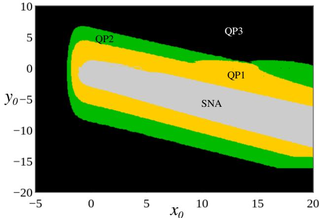
FIG. 3: Basin of attraction for  $f = g = 0.278$ .  $QP1$ ,  $QP2$ , and  $QP3$  are the quasi-periodic attractor-1, quasi-periodic attractor-2, and quasi-periodic attractor-3, respectively. SNA represents the strange nonchaotic attractor. We fixed the other parameter values the same as in Fig. 1.
