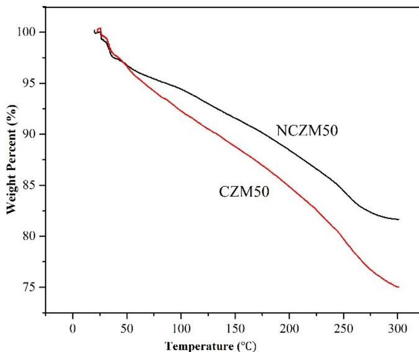
Fig. 4. The TGA result of the NCZM50 and CZM50 samples.
