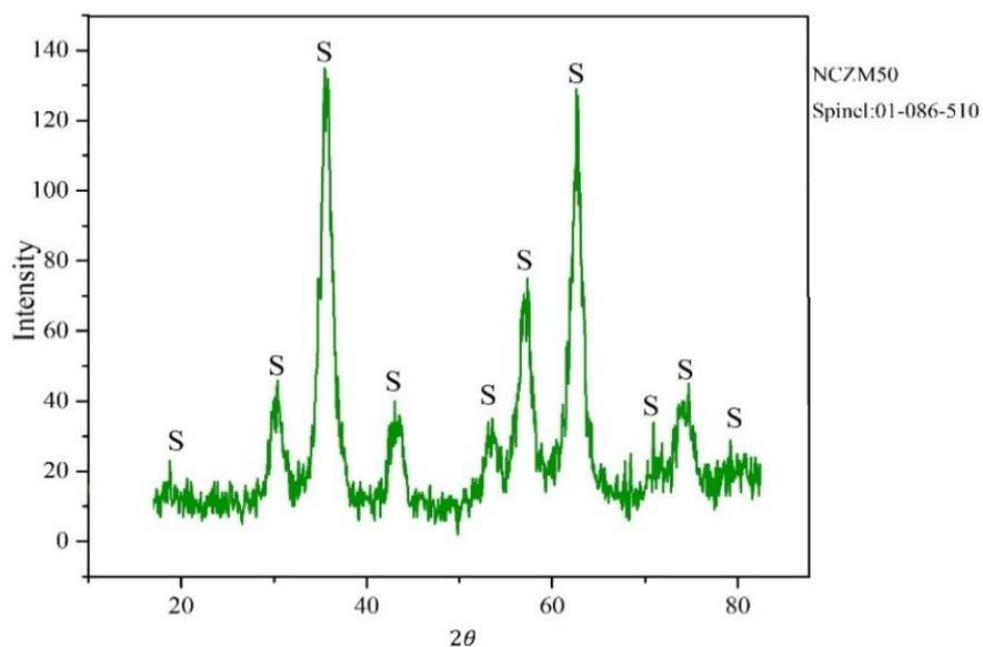
Fig. 2. The XRD pattern of the NCZM50 sample.
