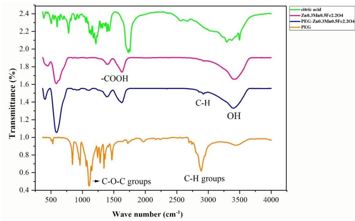
Fig. 3. The FT-IR spectra of the pure NCZM50 and PEG-coated CZM50 NPs along with the PEG coating and citric acid.
