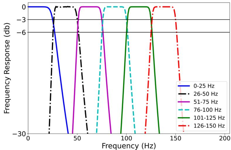
Figure 3. Frequency response of different frequency bandwidths using 7<sup>th</sup> order, zero-phase Butterworth filters
