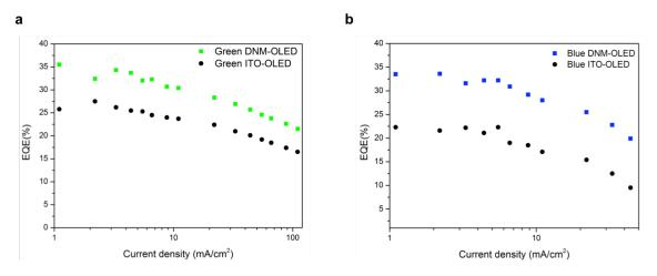
**Figure 7.** Measured EQE of Green and Blue DNM-OLEDs. EQE vs. current density of green (a) and blue (b) DNM-OLEDs. Compared with the ITO-OLLEDs, the maximum EQE of the DNM-OELDs exhibit 1.31-fold enhancement increasing from 26% to 34% for green light and 1.45-fold enhancement increasing from 22% to 32% for blue light.
