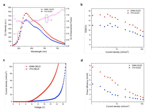
**Figure 4.** Measured electro-luminance (EL), EQE, J-V and power efficiency of DNM-OLEDs and ITO-LEDs. (a) Total front-surface EL/enhancement spectrum; (b) EQE vs. current density; (c) current density vs. driving voltage; (d) power efficiency vs. current density. Compared with ITO-OLEDs, DNM-OLEDs show 1.44-fold average EL enhancement, 1.33-fold max. EQE enhancement, lowered driving voltage by 46% (at 6mA/m<sup>2</sup>) and 1.8-fold max. power efficiency enhancement.
