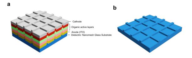
**Figure 1. Dielectric-Nanomesh Organic Light Emitting Diode (DNM-OLED).** (a) The layer structure schematic: a bottom dielectric-nanomesh substrate; anode, organic active layers and cathode deposited on top of it forming a multilayer-corrugated structure; (b) structure schematic of the dielectric nanomesh substrate: a glass substrate with a subwavelength nanomesh etched into it.
