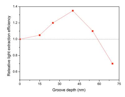
Figure 6. Light extraction efficiency of DNM-OLEDs with respect to the ITO-OLEDs as a function of the groove depth of the dielectric-nanomesh substrate.
