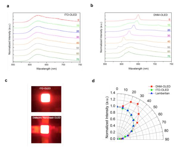
**Figure 5.** Angular-dependent EL spectra, luminance and emission profiles of DNM-OLEDs and ITO-LEDs. (a) normalized EL spectra of ITO-OLEDs (b) normalized spectra of DNM-OLEDs (c) photos of working ITO-OLEDs (upper) and DNM-OLEDs (bottom) indicating the 2D far-field intensity profiles (d) normalized luminance vs. emission angle of ITO-OLEDs and DNM-OLEDs (along the periodic direction of nanomesh).
