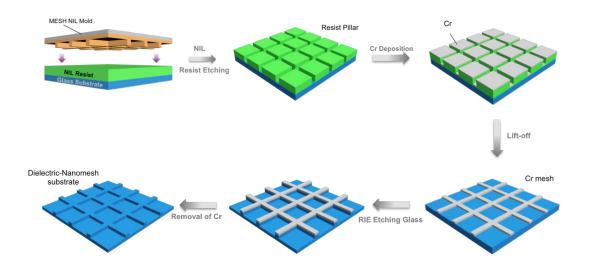
**Figure 2. Fabrication of Dielectric-Nanomesh substrate.** fabrication process: fabrication of Cr nanomesh on a glass substrate by nanoimprint, Cr deposition and lift-off, RIE etching of glass substrate with Cr nanomesh as mask, removal of Cr.
