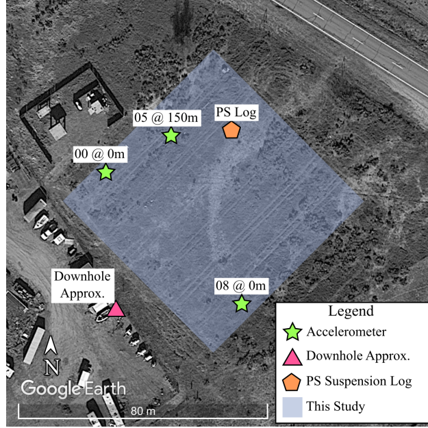
Figure 1: Plan view of the Garner Valley Downhole Array (GVDA) site with the locations of three of the permanent ground motion accelerometers indicated with stars, the approximate location of the seismic downhole test performed by Gibbs (1989) indicated with a triangle, the location of the PS suspension logging performed by Steller (1996) indicated with a pentagon, and the shaded area indicating the region of interest for the present study.
