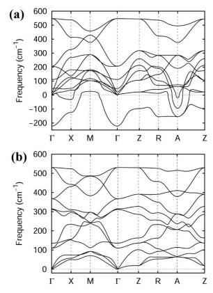
FIG. 3. Phonon spectrum of (a) the nonpolar and (b) the polar  $BiNiO_2$  along the  $\Gamma(0, 0, 0)$ -X(0, 0.5, 0)-M(0.5, 0.5, 0)- $\Gamma$ -Z(0, 0, 0.5)-R(0, 0.5, 0.5)-A(0.5, 0.5, 0.5)-Z directions. The imaginary frequencies are indicated as negative values.
