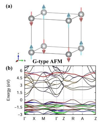
FIG. 9. (a) The G-type of antiferromagnetic (AFM) order. (b) HSE06 band structures of G-type AFM states for a  $\sqrt{2} \times \sqrt{2} \times 2$  supercell in the polar BiNiO<sub>2</sub>. The color has the same meanings as in Fig. 4.
