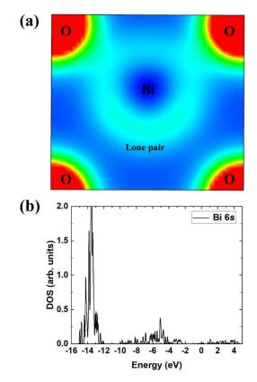
FIG. 6. (a) Electron densities and (b) partial (Bi 6s orbitals) density of states for polar BiNiO<sub>2</sub>.
