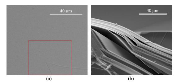
**Figure 3.** The microstructure of the surface of the  $WTe_2$  single crystal: (a) the surface of the (001) type, (b) the lateral surface of the sample. The region in which the chemical composition of the sample was investigated is highlighted in Fig. 3a.
