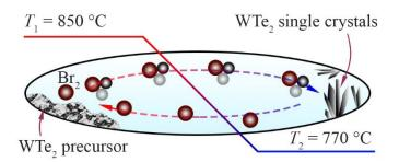
Figure 1. The scheme of growing  $WTe_2$  single crystals by the chemical vapor transport method with  $Br_2$  as a transport agent.
