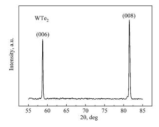
**Figure 2.** A fragment of a diffraction pattern ( $CrK\alpha$ ) taken from the surface of a WTe<sub>2</sub> single crystal.
