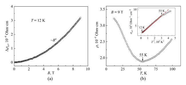
**Figure 6.** (a) The field dependence of the magnetoresistivity  $\Delta \rho_{xx}(B)$  of WTe<sub>2</sub> at T = 12 K. (b) Temperature dependence of the resistivity  $\rho(T)$  of WTe<sub>2</sub> in a magnetic field of 9 T in the temperature range from 12 to 100 K. The inset shows the conductivity  $\sigma_{xx} = f(T^2)$  in a magnetic field of 9 T in the temperature range from 12 to 65 K.
