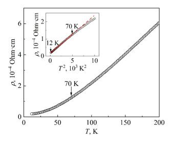
**Figure 5.** The temperature dependence of the electrical resistivity  $\rho(T)$  of WTe<sub>2</sub> in the temperature range from 12 to 200 K. The inset shows the dependence  $\rho = f(T^2)$  in the temperatures from 12 to 100 K.
