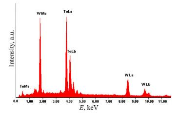
**Figure 4.** Analysis of the chemical composition of the WTe<sub>2</sub> single crystal in the region highlighted in Fig. 3a. The contents of W and Te is are 33.17 and 66.83 at %, respectively.
