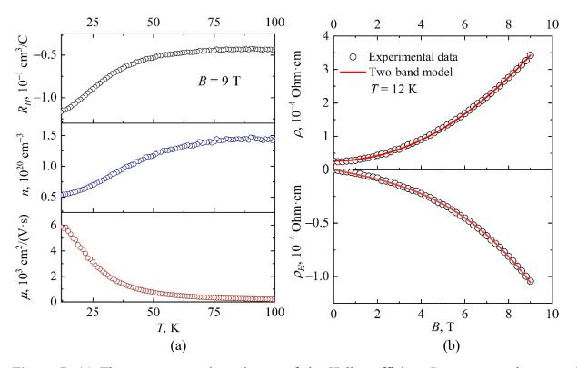
**Figure 7.** (a) The temperature dependences of the Hall coefficient  $R_{\rm H}$ , concentration *n*, and mobility  $\mu$  of current carriers in WTe<sub>2</sub> according to a single-band model in a magnetic field of B = 9 T. (b) Field dependences of resistivity  $\rho(B)$  in the magnetic field and Hall resistivity  $\rho_{\rm H}(B)$  for WTe<sub>2</sub> at T = 12 K: open circles show the experimental data; the solid red lines are curves obtained within the framework of the two-band model.
