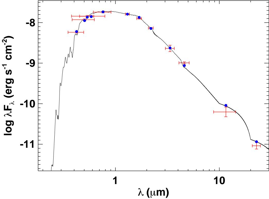
**Figure 2.** Spectral energy distribution of HD 76920. Red symbols represent the observed photometric measurements, where the horizontal bars represent the effective width of the passband. Blue symbols are the model fluxes from the best-fit Kurucz atmosphere model (black).
