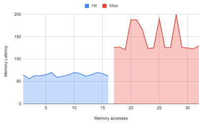
Fig. 4. Latency measured by threaded timer showing enough resolution to distinguish hit from miss
