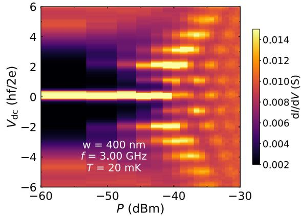
Figure S11: **a**, Color mapping of  $dI/dV$  measured in Junction 1 on a TI ribbon with  $w = 400$  nm under rf irradiation at frequency  $f = 3$  GHz as a function of rf power  $P$  and applied dc voltage  $V_{\text{dc}}$  at  $B = 0$  T and  $T = 20$  mK.
