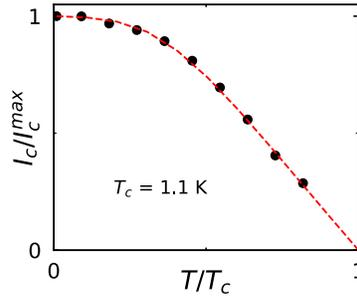
Figure S9: Temperature dependence of  $I_c$  in Junction 1 obtained from  $dV/dI$  vs  $I_{dc}$  at various temperatures up to 0.9 K. The red dashed line is the behavior of the theoretical formula given by Galaktionov and Zaikin<sup>10</sup> with  $T_c \approx 1.1 \text{ K}$  and transparency  $\mathcal{T} \approx 0.5$ .
