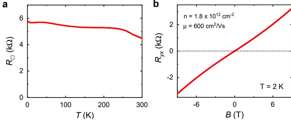
Figure S8: **a**, Temperature dependence of the sheet resistance  $R_{\square}$  of the pristine BST film used for the Josephson Junctions 2 and 3 used for Figs. 3d, 4c, and 4d of the main text. **b**, Hall resistance  $R_{yx}$  as a function of magnetic field  $B$  of the same thin film.
