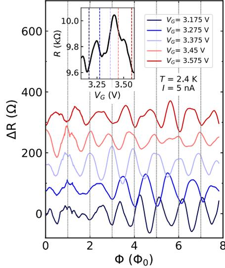
Figure S6: **a**, Resistance change  $\Delta R$  as a function of magnetic flux  $\Phi$  (in units of the flux quantum  $\Phi_0$ ) at selected  $V_G$  positions showing  $\pi$ -phase shifts in the oscillations. Inset shows the positions of the selected  $V_G$  values in relation to the  $R(V_G)$  behavior near the CNP.
