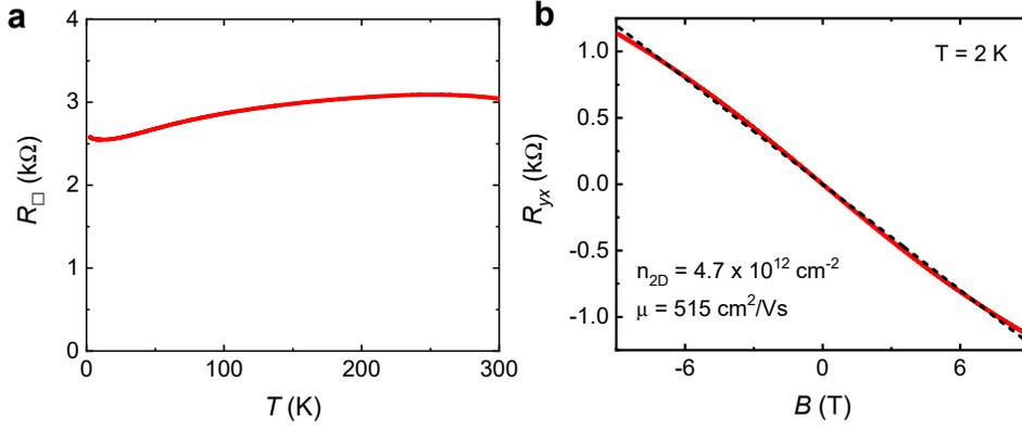
Figure S2: **a**, Temperature dependence of the sheet resistance  $R_{\square}$  of the pristine BST film used for the 500-nm-wide Hall-bar device discussed in the main text. **b**, Hall resistance  $R_{yx}$  as a function of magnetic field  $B$  of the same thin film.
