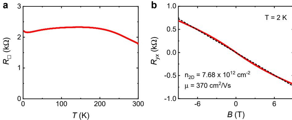
Figure S3: Temperature dependence of the sheet resistance  $R_{\square}$  of the pristine BST film used for the gate-tunable Device 1 used for Fig. 1g and Fig. 2 of the main text. **b**, Hall resistance  $R_{yx}$  as a function of magnetic field  $B$  of the same thin film.
