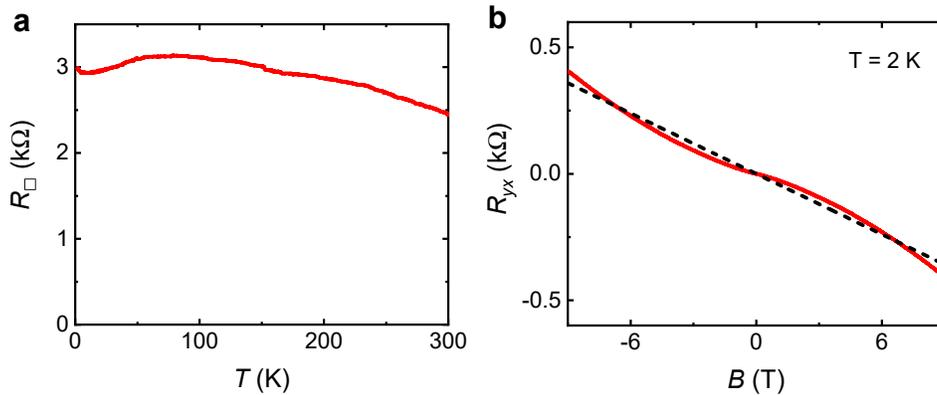
Figure S7: **a**, Temperature dependence of the sheet resistance  $R_{\square}$  of the pristine BST film used for the Josephson junction 1, whose results are shown in Figs. 3b, 3c, 4a, and 4b of the main text. **b**, Hall resistance  $R_{yx}$  as a function of magnetic field  $B$  of the same thin film.
