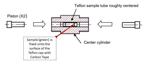
**Figure S1** Depiction of the center cylinder and pistons of the BeCu pressure cell. Inside the center cylinder is a Teflon tube with Teflon caps on each end.
