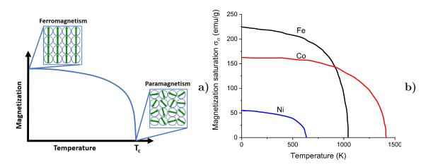
Figure 1.3: a) Change of the magnetic ordering from ferro- to paramagnetism with increasing temperature up to the Curie temperature  $T_C$ ; b) Finite temperature magnetization curves for the elements Fe, Co and Ni up to their  $T_C$ 's of 1044, 1388 and 628 K. Image b) is based on data from [6].
