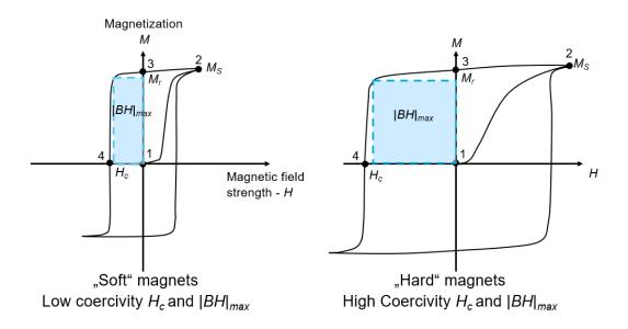
Figure 1.1: Hysteresis loop for soft (left) and hard (hard) magnetic materials. Important magnetic properties like the magnetization saturation  $M_S$  are marked and the maximum energy product  $|BH|_{max}$  is depicted as a blue square in the second quadrant.
