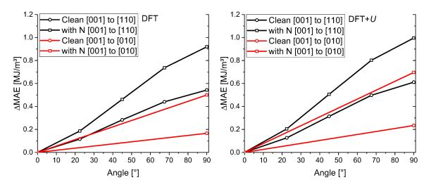
Figure 5.8: Calculated energy differences of the magnetocrystalline energy for the shift of the crystallographic direction from [001] to [110](black) and [100] to [010] (red) for the clean (circles) and nitrogenated (squares) NdFe<sub>11</sub>Ti compound. On the left side are DFT and on the right side DFT+U results shown. For the change from [001] to [110] the angles 0, 22.5, 45, 67.5 and 90° are considered. For the change from [001] to [010] only the 0 and 90° angles are considered.
