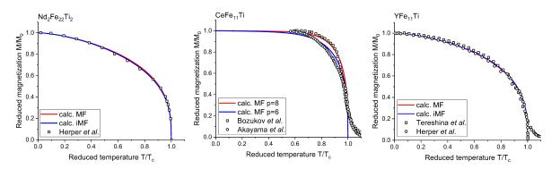
Figure 5.7: Finite temperature magnetization calculated on basis of the Körmann and Kuzmin approaches. For comparison the experimental data by Herper *et al.* [75], Bozukov *et al.* [108], Akayama *et al.* [81] and Tereshina *et al.* [80] are shown. For the NdFe<sub>11</sub>Ti and YFe<sub>11</sub>Ti compounds the Kuzmin and the Körmann approaches are used. For the CeFe<sub>11</sub>Ti compound the Kuzmin approach with p=8 (red) and p=6 (blue) are depicted.
