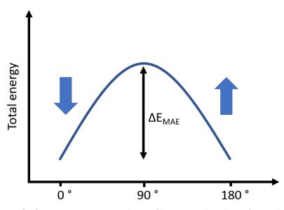
Angle between easy axis and magnetization direction
