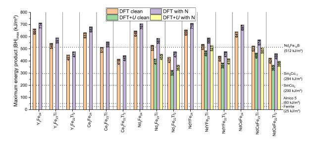
Figure 5.5: Theoretical maximum energy product  $|BH|_{max}$  values for considered compounds and nitrogenated cases. In addition to conventional DFT, DFT+U with U=6 eV has been considered for stable Nd-contained alloys. Experimental values [10, 101] of most common hard magnets are given as horizontal dotted lines.
