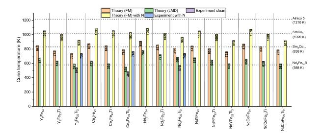
Figure 5.6: Calculated Curie temperatures  $T_{\rm C}$  for the clean and nitrogenated 1:12 phases. Exchange interaction energies have been calculated with both ordered ferromagnetic (FM) and disordered local moment disorder (LMD) states, and the input lattice information is taken from our theoretically relaxed calculations (check Tab. 5.1). Experimental data is taken from [86, 104].
