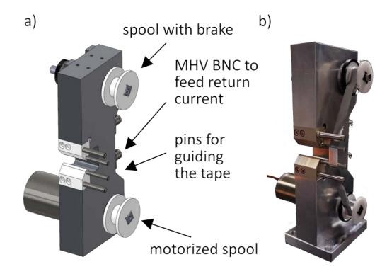
Figure 1. Tape target system for petawatt shots at VEGA-3: (a) technical details in the CAD illustration such as (i) the spool running over a break; (ii) the motorized spool; and (iii) the grounding pins keeping the tape in focal position; and (b) a photograph of the system. Note that pins are conductively connected to the ground via the MHV BNC connection in order to ensure grounding.
