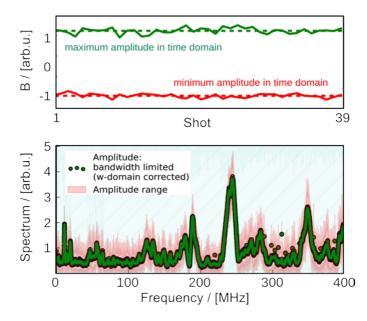
Figure 6. The maximum and minimum magnetic-field amplitude of the time-domain signal (top) and the time integrated average magnitude spectrum (bottom) of **39** shots with the same laser parameters of  $(28.5 \pm 0.3)$  J pulse energy and  $(31 \pm 2)$  fs pulse duration on Tape 9-Al-e-K.
