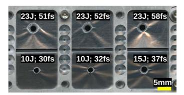
Figure 10. After the laser shot evaporated target material gives way to an ablation hole in the  $9\,\mu m$  thick Aluminium tape, the  $125\,\mu m$  thick Mylar layer that was pressed onto the Aluminium does not show clear signs of ablation.
