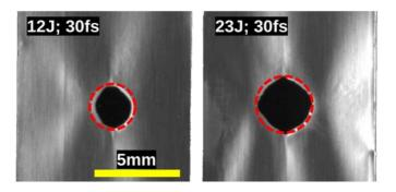
Figure 8. After the laser shot evaporated target material gives way to an ablation hole in the  $9 \mu m$  thick Aluminium tape, (left) for 12 J and (right) for 23 J laser pulse energy at best compression. Dashed lines indicate perfect circles (the circle on the right side is larger than the circle on the left side).
