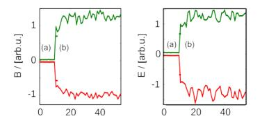
Figure 7. The maximum and minimum amplitude of the time-domain signal (left) for magnetic-fields and (right) for electric-fields of one run with shots on Tape 9-Al-e-K. Pulse energy and pulse duration vary from 2028 and  $(31 \pm 2)$  fs. Shots (a) are biased by miss-alignments and shots (b) show sensitivity to laser parameters.
