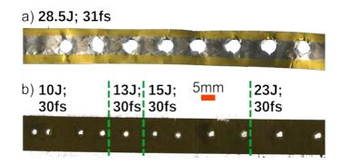
Figure 4. Tape types used during the experiment, respectively scanned after laser shots indicated with their laser pulse parameters. (a) Tape 9-Al-e-K with a mm-thin stripe sticked on each edge, and (b) Tape 89-K-l-ad pure Kapton tape with Silicon Adhesive on the rear side. (a) and (b) have the same scale.
