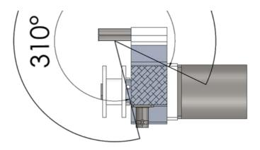
Figure 2. Top-view with a horizontal cut through the tape target system, with indication of the range that allows free field of view onto the interaction point on the tape.
