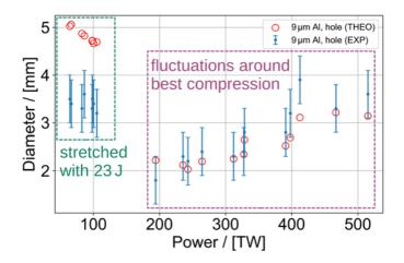
Figure 9. The diameter of the evaporation hole on a  $9 \mu m$  thick Aluminium tape under variation of the laser pulse power at best focus, compared are experimental results (EXP) and theoretical predictions (THEO). Highlighted are two groups of shots, (green) at 23 J of laser power under variation of the laser pulse duration-, and (purple) around best compression under variation of the laser pulse energy.
