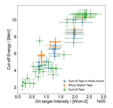
Figure 5. The spectral cut-off energy of accelerated proton beams is recorded for a fixed focal spot size but under variation of laser pulse energy and duration for three types of tape.
