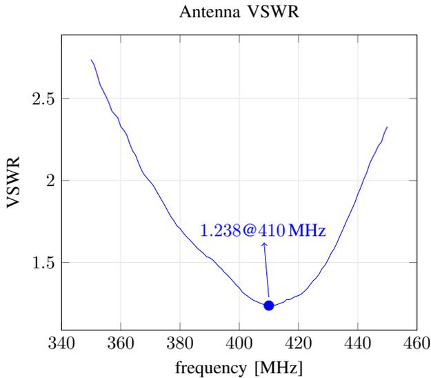
Fig. 5: VSWR graph - antenna analysis between 350 and 450 MHz.
