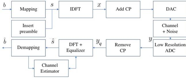
Fig. 1: Block diagram of the proposed Q-OFDM system.
