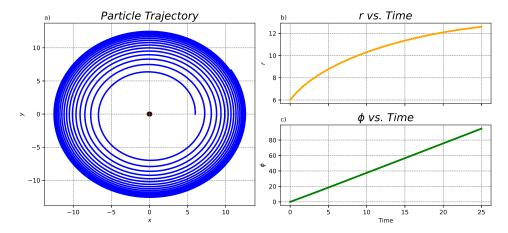
Figure 2: Trajectory of a particle with mass m=1, around a black hole with mass M=1. The initial conditions are  $r_0=6$ ,  $\phi_0=0$ , the particle energy is  $E=-\sqrt{8/9}$ , the angular momentum is  $j=\sqrt{12}$  and the spin is s=3.
