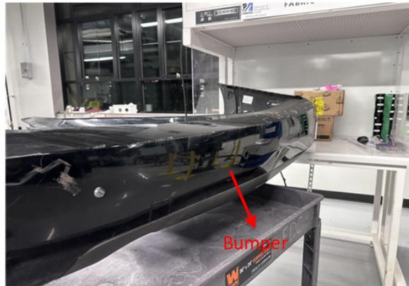
**Supplementary Figure 5. Photos of the printed flexible radar which is conformally integrated with a vehicle rear bumper.**
