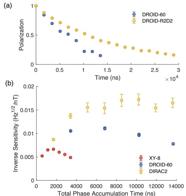
FIG. 3. **Experimental improvements for dynamical decoupling and sensing with higher-order pulse sequence design.** (a) Experimental coherence decay curves under dynamical decoupling with different sequences, where the new sequence DROID-R2D2 significantly outperforms the existing sequence DROID-60. (b) Experimental AC magnetic field sensitivities, where our new sequence DIRAC2 is significantly better than DROID-60 and XY-8, improving quantum sensing with strongly-interacting spin ensembles.
