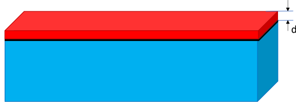
Figure 4. A metallic (N) layer of thickness d (red) coupled by the proximity effect to the bulk superconducting (S) substrate (blue). The black layer between N and S depicts a resistive interface barrier.
