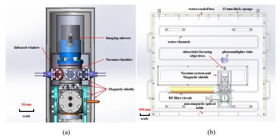
Fig. 2. (a) The vacuum chamber is made of titanium alloy to avoid the magnetic field produced by the
