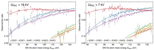
**Figure 6.** Ratios of the best-fit relative response function obtained from the model compared with the observed rate ratios as a function of incoming ISN helium atom mean energy. The observed rate ratios are binned in 1-eV-wide energy bins. The left and right panels show results for a PAC voltage of 16 and 7 kV, respectively.
