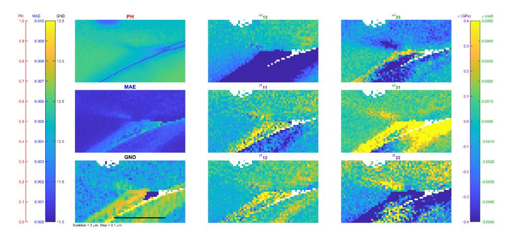
Figure 12 - HR-EBSD analysis of the pinched off hydride map – Tip 1
