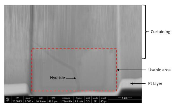
Figure 18 - pFIB hydride area overview. SE image showing the polished hydride region, with the useable area indicated by the red dashed box and the start of significant curtaining indicated. Scalebar =  $5 \mu m$ .
