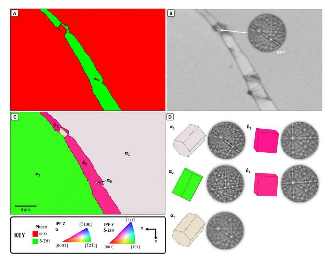
Figure 2 – Orientation analysis of the grain boundary hydride map: (A) Indexed phase map; (B) pattern quality map (with probable SPP representative pattern); (C) crystal orientation (IPFZ coloured) along with labels for key grains; (D) prisms and representative patterns for the identified grains. Figure 2 shows an overview of the orientations in the grain boundary hydride map. From
