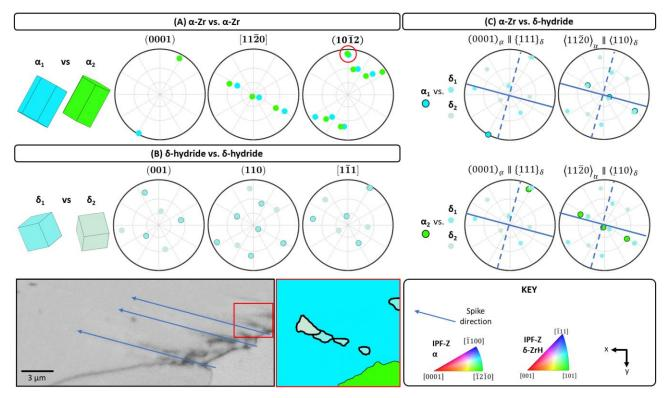
Figure 15 - Orientation relationships in the spiky hydride map. Pole figure analysis of (A)  $\alpha$ -Zr/ $\alpha$ -Zr OR;(B) hydride/hydride OR; (C)  $\alpha$ -Zr/ $\delta$ -hydride OR. (D) Pattern quality map with hydride directions annotated; (E) Zoomed in orientation map (IPFZ colouring) showing the two hydride orientations within a hydride spike.
