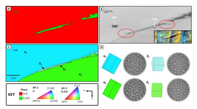
Figure 9 - Orientation analysis of the pinched off hydride map.(A) Indexed phase map; (B) pattern quality map with SPPs indicated and red ovals highlighting the pinched off sections of hydride (insert: forescatter image of the hydride); (C) crystal orientation (IPFZ coloured) along with labels for key grains; (D) prisms and representative patterns for the identified grains.
