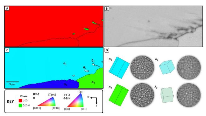
Figure 14 - Orientation analysis of the spiky hydride map. (A) Indexed phase map; (B) pattern quality map; (C) crystal orientation (IPFZ coloured) along with labels for key grains; (D) prisms and representative patterns for the identified grains.
