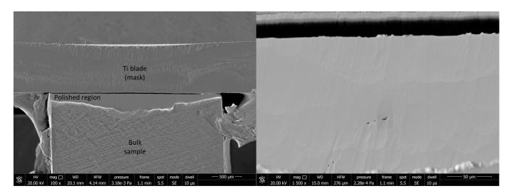
Figure 19 – BIB cross-sectioned surface. (A) Secondary electron (SE) image showing the location of polished region whilst sample is attached to Ti blade that acts as a mask during cross-sectioning. (B) higher magnification SE image of the polished region showing some localised surface roughness.
