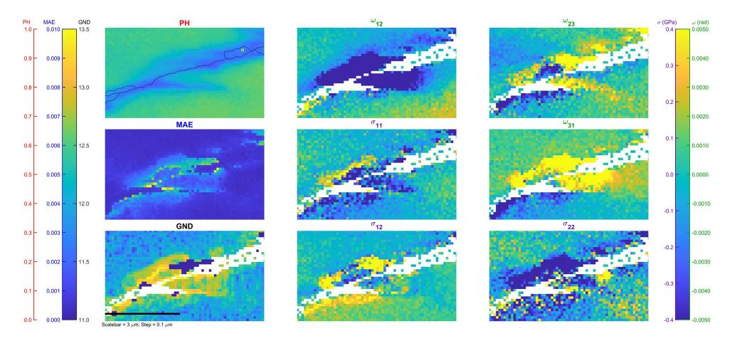
Figure 13 - HR-EBSD analysis of the pinched off hydride map – Tip 2
