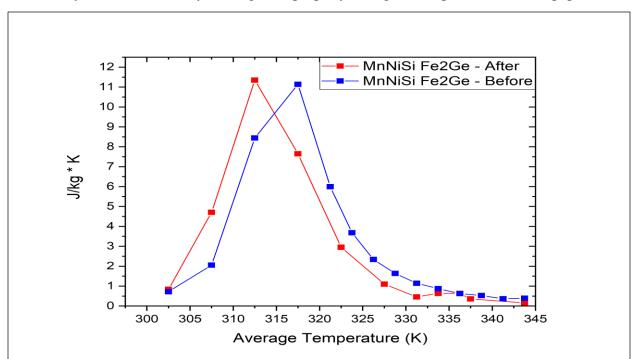
Fig. 5 Magnetic entropy change for a magnetic field change of 3 T before irradiation (blue) treatment of  $(MnNiSi)_{1-x}(Fe_2Ge)_x$ , where x = 0.34 and magnetic entropy change curve after irradiation (red) treatment of  $(MnNiSi)_{1-x}(Fe_2Ge)_x$ , where x = 0.34
