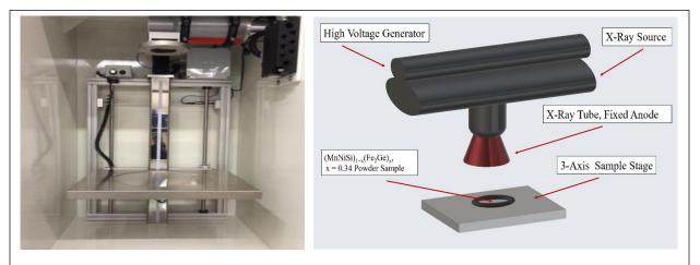
Fig 1. Experimental setup of the X-rad 225 XL for irradiation treatment of  $(MnNiSi)_{1-x}(Fe_2Ge)_x$ , where x = 0.34
