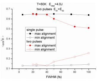
Fig. 3. The optional alignment and anti-alignment of O2 molecules under one pulse (black line) and two pulses (red line) at the same input energy.
