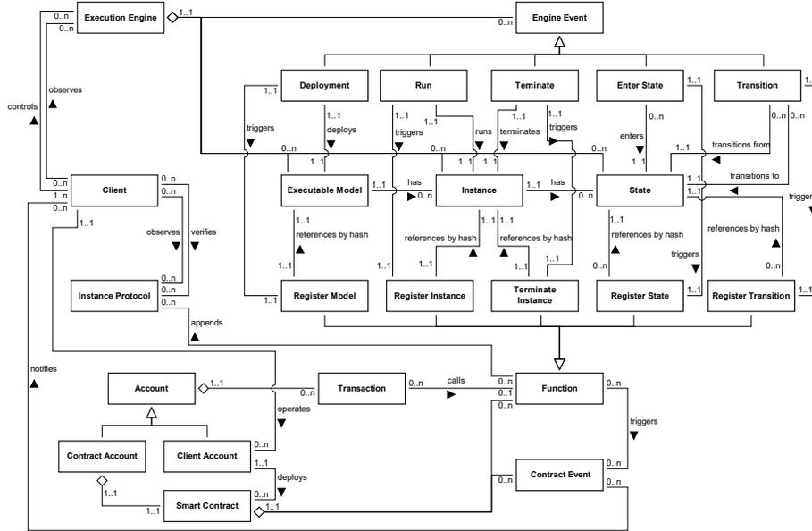
**Fig. 1.** Metamodel describing the concepts for model-based execution and instance tracking. Clients exercise control over an execution and observe models with instances and states through the events of a smart contract.
