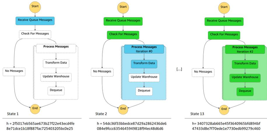
**Fig. 4.** AWS Step Functions instance created from the model shown in Figure 3. The instance consists of 13 states for parallel data processing, executed in multiple concurrent iterations. By chance, the last state of the instance belongs to "Iteration #2".
