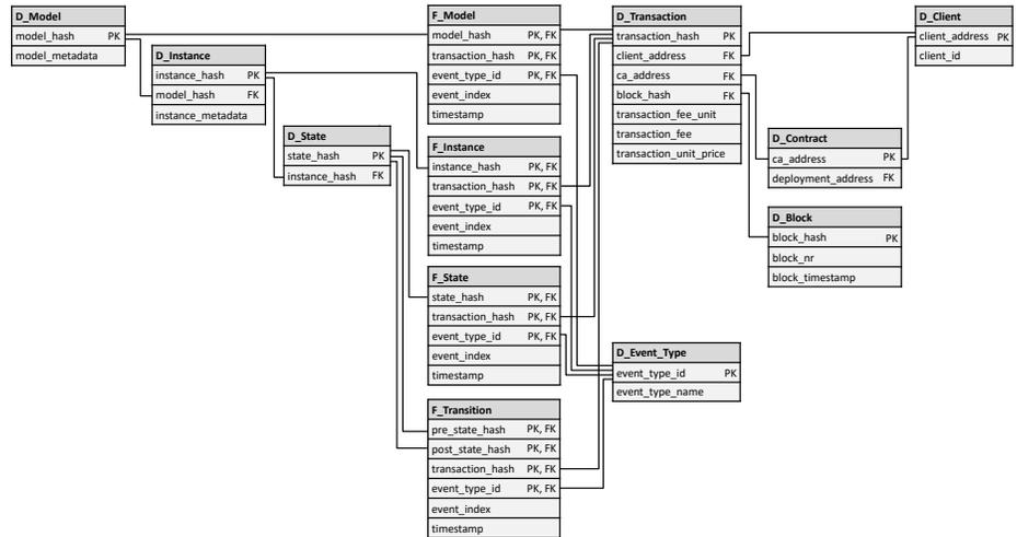
**Fig. 2.** Multidimensional data model for tracking models, instances, states, and transitions according to smart contract events. Tracking and aggregation is supported over dimensional data (prefix D), e.g. for clients or contracts, for the events stored as fact data (prefix F).
