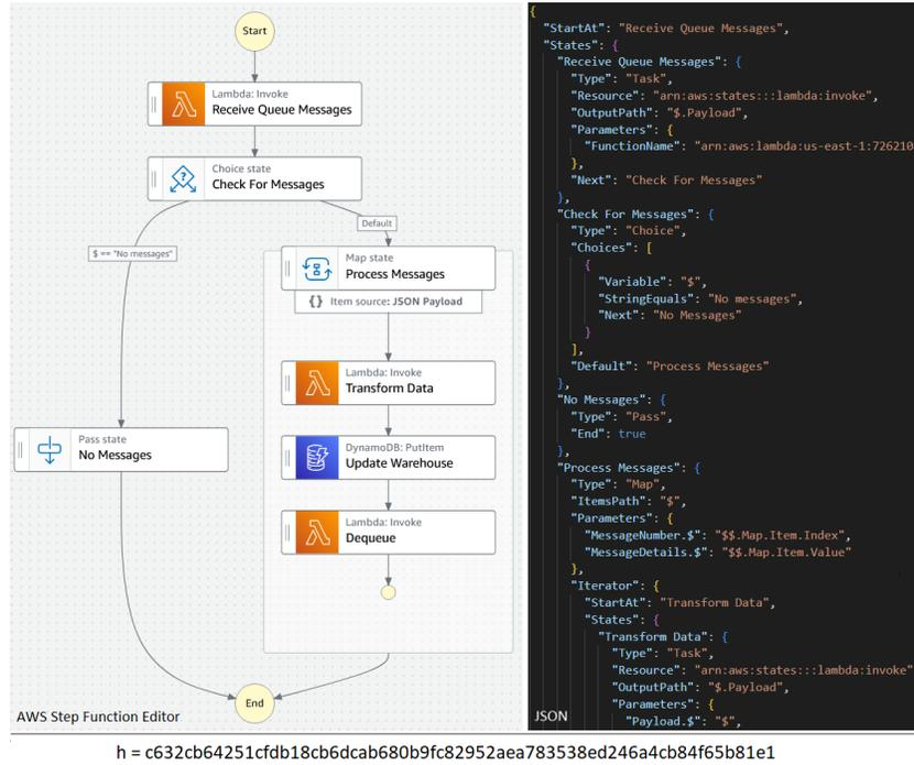
**Fig. 3.** AWS Step Functions model for parallel data processing in a distributed scenario, where data is received through a message queue, transformed, and stored in a data warehouse. The model is shown as state machine diagram and JSON representation. A hash value  $h$  is used for identification based on the model content and for verification.
