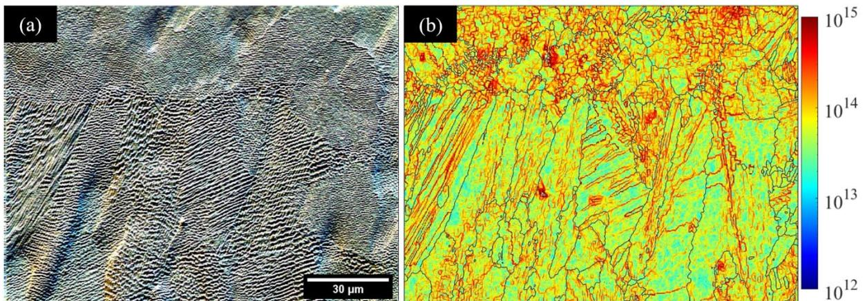
Figure 5. GNDs located at and aligned along the boundaries of cells (or dendrites): (a) SEM micrograph showing the cellular arrays in as-built Inconel 718; (b) corresponding GND spatial distribution map.
