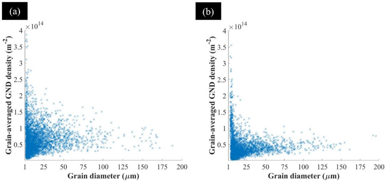
Figure 6. GND density as a function of grain diameter in the as-built and undeformed (a) B0 condition and (b) CB67 condition. The data was measured from the top-view maps.
