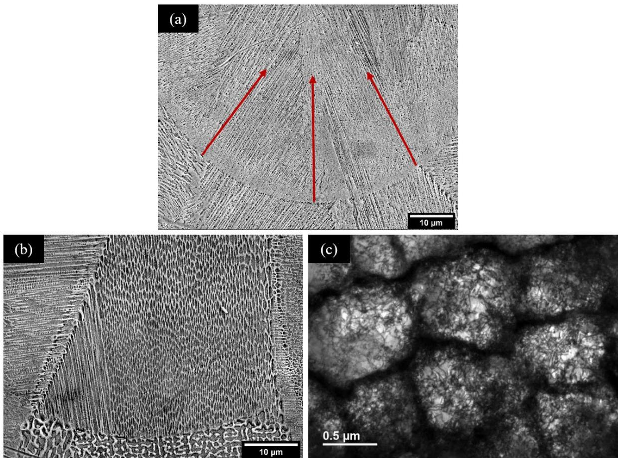
Figure 2. As-built microstructure of Inconel 718 processed by L-PBF. (a) Microstructure in a deposition bead with arrows showing the growth direction of cells that were initially almost perpendicular to the fusion boundary. (b) Side-branching across the fusion boundary was seen in the top left region. (c) Cells containing a high density of dislocations, particularly at the cell boundaries.
