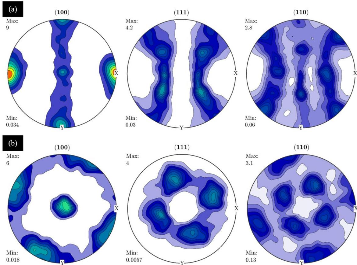
Figure 4. Pole figures of the (a) B0 condition and (b) CB67 condition. Data acquired from the top-view maps. X and Y are perpendicular to the building direction. X is parallel to the longitudinal axis of the samples, which is along the B0 scanning bi-directions, whereas Y is perpendicular to this axis.
