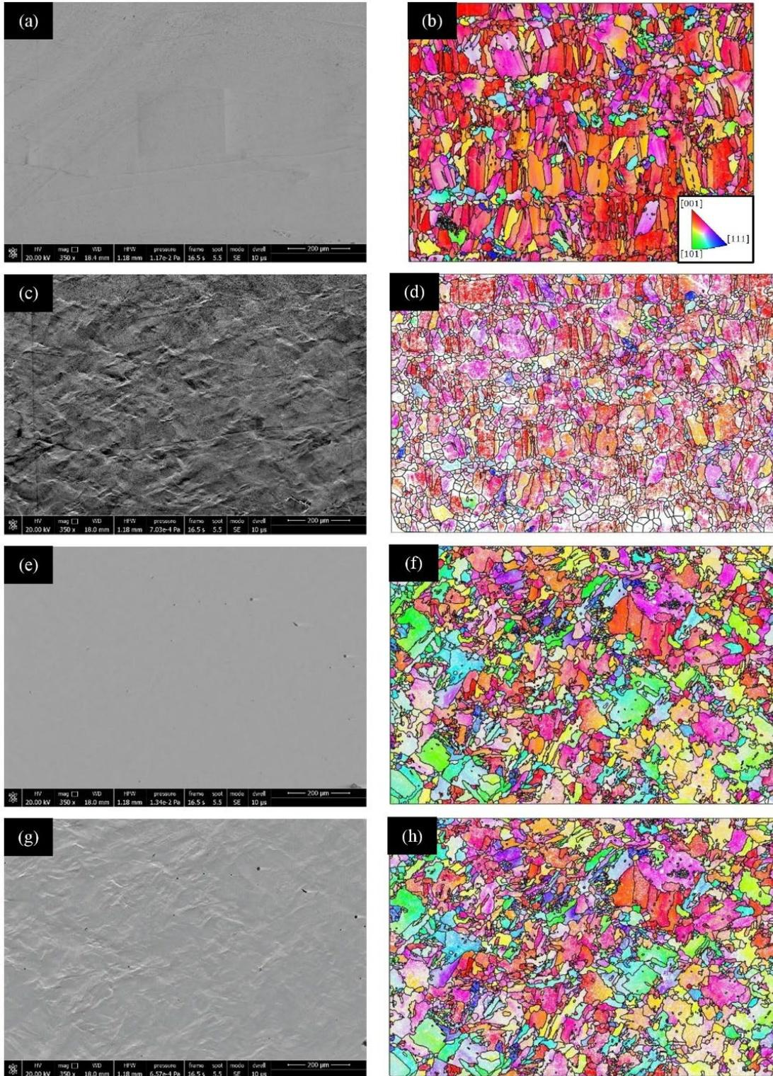
Figure 10. SEM images and their corresponding IPF maps along the loading direction for (a-b) undeformed B0 condition; (b-c) deformed B0 condition at 10% strain; (e-f) undeformed CB67 condition; (g-h) deformed CB67 condition at 10% strain. All figures have the same scale bar.
