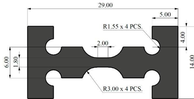
Figure 1. *In-situ* testing sample geometry. All dimensions in mm and figure not to scale.
