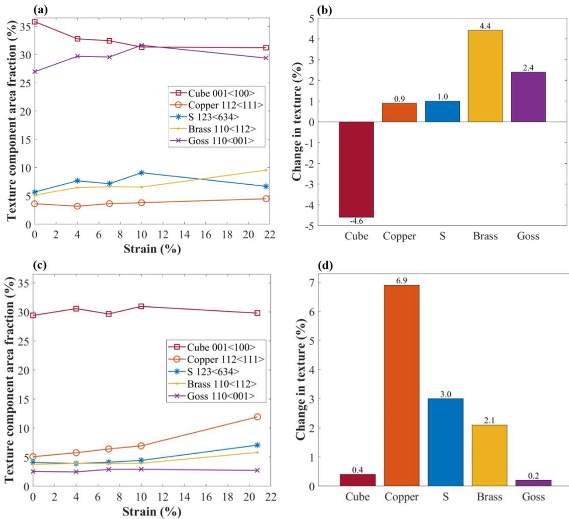
Figure 11. Evolution of texture component area fraction across the strain intervals and their overall change from the as-built to fractured: (a-b) B0 condition and (c-d) CB67 condition.
