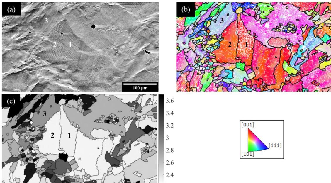
Figure 8. Slip transmission across neighbouring grains in the CB67 condition at 10% strain. All figures are of the same region: (a) SEM image; (b) EBSD-IPF along the loading direction; (c) Taylor factor map.
