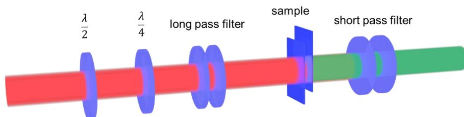
*Figure S2.* The optical path for SHG measurement.  $\lambda/2$  and  $\lambda/4$  represent the half-wave plate and quarter-wave plate, respectively.
