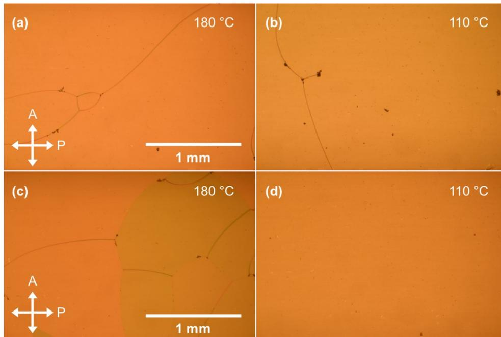
*Figure S1.* The PLM texture of two HN\* in a 50  $\mu\text{m}$  thickness cell. a) and b) the texture of 1.1%R811/RM734 at 180 °C and 110 °C , respectively; c) and d) the texture of 1.1%S811/RM734 at 180 °C and 110 °C, respectively. The scale bar is 1 mm.
