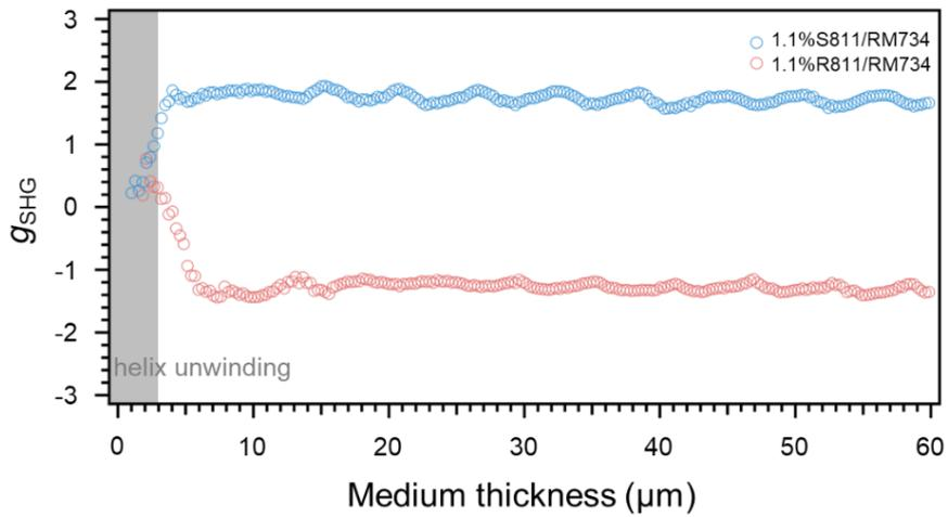
*Figure S3.* The thickness dependencies of the  $g$ -factor of right-handed HN\* 1.1%R811/RM734 and left-handed HN\* 1.1%S811/RM734, respectively. The gray part indicates the thinnest part of the wedge-shaped cell (0~3  $\mu\text{m}$ ), where the polarization field is in the unwinding state, and the SHG-CD effect is neglectable. Also, some defects are seen in this area, causing some fluctuations of  $g$ -factor.
