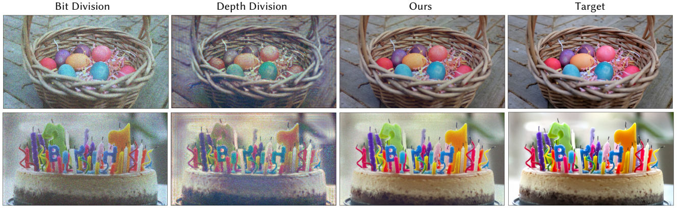
Fig. 5. Comparison of bit division, depth division and our method of simultaneous color holography in simulation. Bit division (Col. 1) is noisier than our method (Col. 3) but achieves comparable color fidelity, although more washed out. The depth division method (Col. 2) is also noisier than our method and has inferior color fidelity. Our method matches the target image (Col. 4) well. Our method uses our perceptual loss function and a high order angular spectrum propagation model with no learned components. Further implementation details for each method are available in the supplement.
