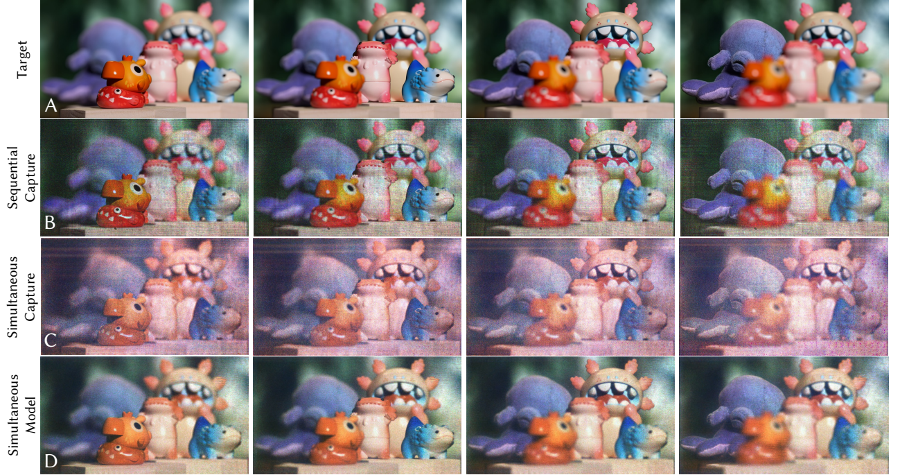
Fig. 7. Experimentally captured focal stack. This figure displays a focal stack, with the target shown in (A), captured from 90 mm to 120 mm in 10 mm increments. We compare (B) the sequential pseudo-color experimental capture with (C) the experimental capture of the simultaneous full color hologram and (D) the simulated model output for simultaneous color. Although model mismatch creates some deviations between the simultaneous capture (C) and the target (A), the simulated model (D) is representative of the color fidelity we expect from our method with improvements to the system calibration.
