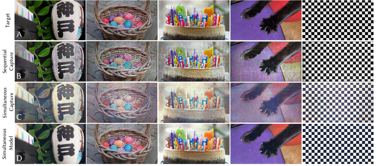
Fig. 6. Experimentally captured 2D holograms. For each target image (A), we show (B) the experimental capture with sequential pseudo-color, (C) our experimental capture with full simultaneous color, and (D) the simulated model output for simultaneous color. Recall that our simultaneous color results (C) use 3\times fewer degrees of freedom than the sequential capture (B). Although some color fidelity is lost in experiment (C), the simulated model output (D) shows good color quality, demonstrating that accurate color is possible with our method and improvements to the calibration.
