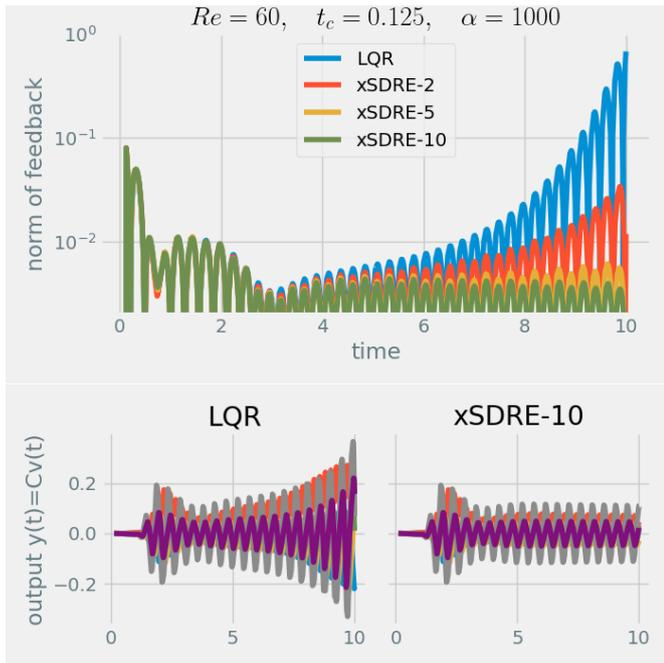
Figure 2: Norms of feedback for different  $r$  and the corresponding outputs for the LQR and the  $\text{xSDRE-10}$ -feedback for the case of  $\alpha = 10^3$  and  $t_c = 0.125$ . A continuous performance improvement for  $\text{xSDRE-r}$  can be observed with stabilization of the system at  $\text{xSDRE-10}$ , while the classical LQR-feedback fails.
