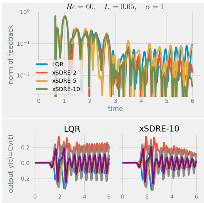
Figure 3: Norms of feedback for different  $r$  and the corresponding outputs for the LQR and the  $\text{xSDRE-10}$ -feedback for the case of  $\alpha = 1$  and  $t_c = 0.65$ . The  $\text{xSDRE-10}$ -feedback is able to stabilize the system in contrast to the classical LQR approach.
