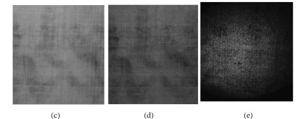
Figure 3: (a) Image of a replica painted over papyrus (Original copy), (b) the chosen region, (c) image under incoherent light illumination, copy turned over, (d) as seen in near infrared light and (e) under laser illumination (unprocessed speckle image).
