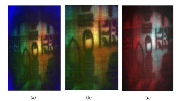
Figure 4: (a) Component R with AVD ( $\phi = 5$ ) in red laser light. Component G with AVD ( $\phi = 5$ ) in green laser and component B corresponds to Tuneable  $\tau$  ( $\phi = 80$ ) blue laser; (b) cut-out and enlargement of Fig. 4 a) and (c) pseudo coloured version with AVD ( $\phi = 0$ ), processed with red laser and exponent LUT  $\alpha=1$ .
