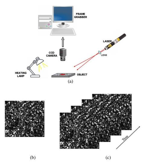
Figure 2: (a) Experimental set-up. (b) speckle pattern of a single frame. (c) stack of successive speckle frames
