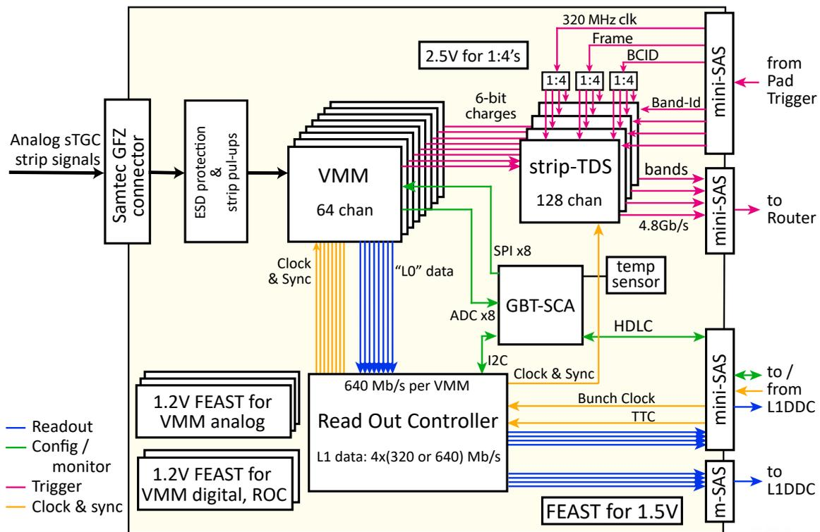
**Figure 20:** Block diagram of the sTGC strip Front-end board that handles the strips in one sTGC gas gap, showing its ASICs, connectors and power blocks. The second MiniSAS connector is used only for the inner quadruplet.
