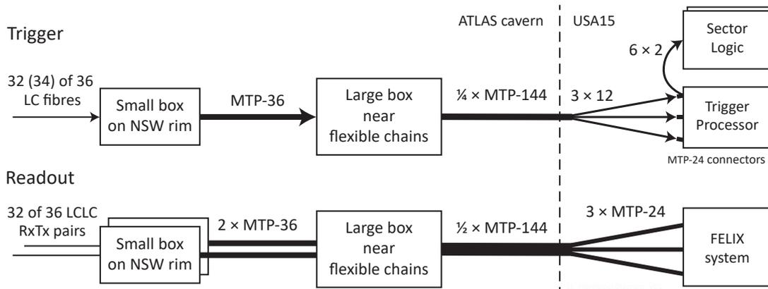
**Figure 28:** Block diagram of the trigger and readout fibre paths for one sector of sTGC or Micromegas. Micromegas has 32 trigger inputs to the Small box, whereas sTGC has two additional inputs from the Pad Trigger for 34 inputs. Six output pairs of the sTGC Trigger Processor are used to fan out the segments to up to seven different Sector Logic sectors. When seven are required, a second Trigger Processor MTP-24 IO connector is used.
