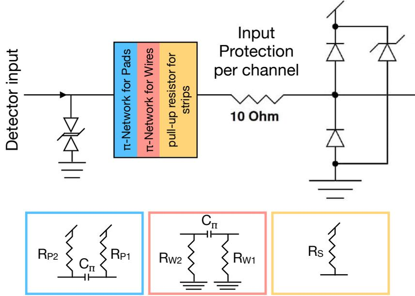
**Figure 19:** The sTGC FEB analog input circuit which protects against transients and compensates for high rate and high charge signals for pads (blue, left), wires (red, middle) and strips (yellow, right).
