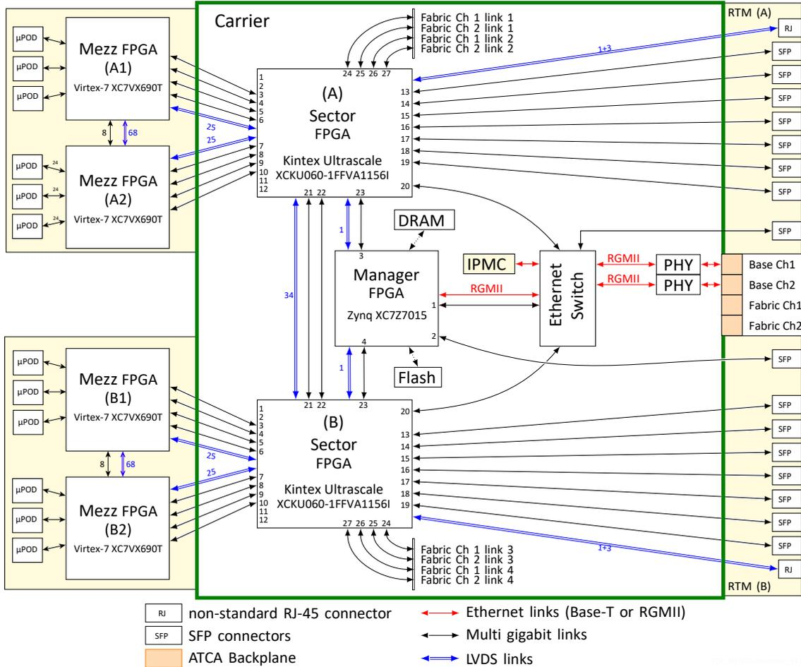
**Figure 6:** Block diagram of the Trigger Processor ATCA card showing the Carrier, two mezzanines, the Rear Transition Module (RTM) and an Intelligent Platform Management Controller (IPMC) card. Each mezzanine hosts an sTGC FPGA and a Micromegas FPGA for a sector.
