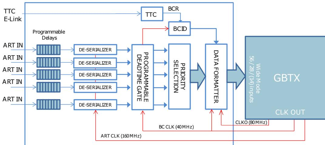
**Figure 16:** Block diagram of the ART ASIC
