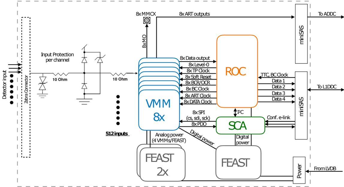
**Figure 18:** The MMFE8 block diagram showing the ESD protection, the VMM Front-end ASICs, the Readout Controller ASIC, the Slow Control Adapter ASIC, the FEAST DC-to-DC converter ASICs, and the MiniSAS twin-ax connectors for the different interfaces.
