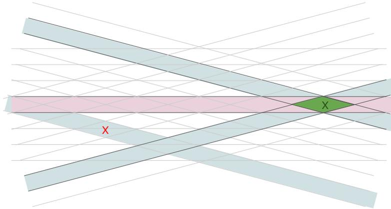
**Figure 9:** Illustration of the Micromegas XUV trigger candidate. The X-plane candidate is merged with the UV-candidate to form a coincidence on the so-called diamond road which corresponds to the geometrical coincidence of the strips.
