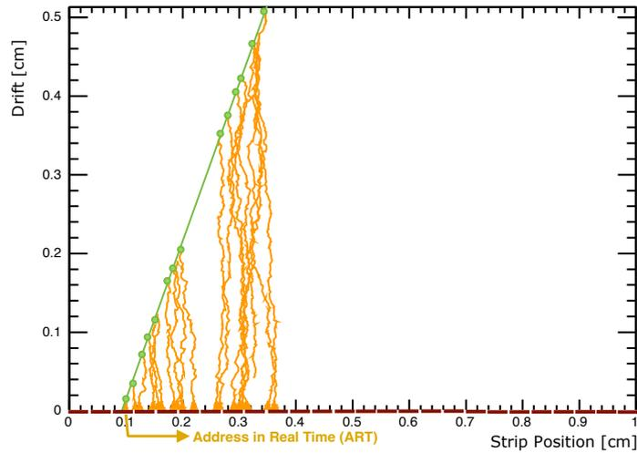
**Figure 3:** A simulated event showing the ionisation from a particle crossing the Micromegas detector at an angle. The address of the strip to which the charge arrives first is output as an ART signal [28].
