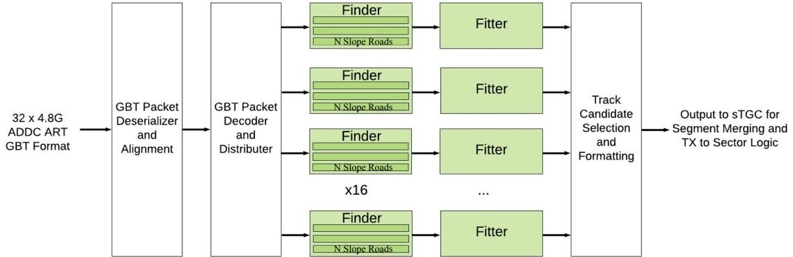
**Figure 8:** The Micromegas Trigger Processor block diagram.
