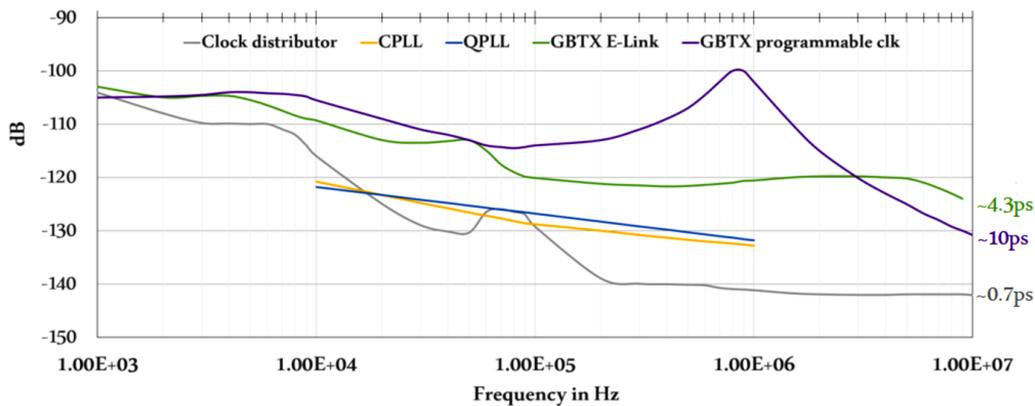
**Figure 27:** Phase noise (random-rms) jitter of the direct and GBTx clocks compared to Xilinx’s phase noise mask for the CPLL and QPLL. The integrated bandwidth for GBTx E-link and programmable clocks is 1 kHz to 20 MHz. The integrated bandwidth for the clock distributor is 1 kHz to 30 MHz [107].
