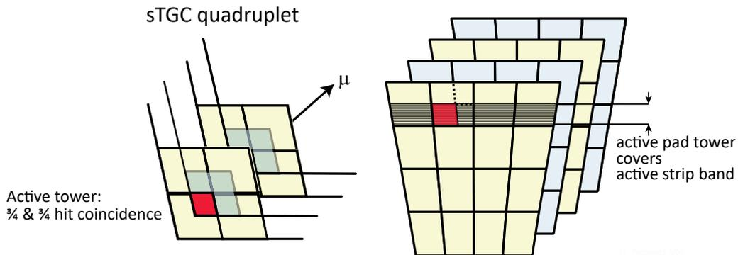
**Figure 2:** A band of strips in each layer is selected by a particle making a 3-out-of-4 hit coincidence in a pointing tower of sTGC pads in each quadruplet. The pads in half of the layers are shifted by half a pad in both directions to increase the resolution. Eight-layer towers pointing to the interaction point are defined by the overlapping physical pads (shown in grey) which identify a logical pad (in red) in each layer.
